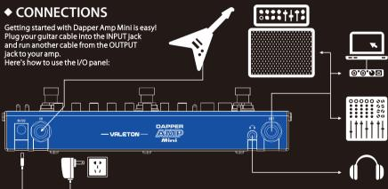
Note: 1. If Dapper Amp Mini sounds harsh or weird when connecting to the input jack on your amp, try connecting to the amp's FX Loop return jack.
